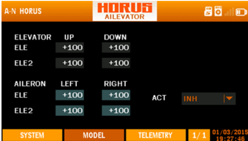
Overview of the ailevator menu screen
