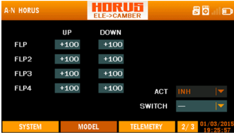
Overview of the elevator->camber 2/3 menu screen
