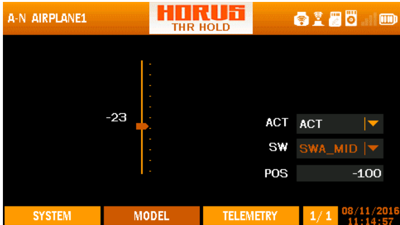
Overview of the throttle hold menu screen
