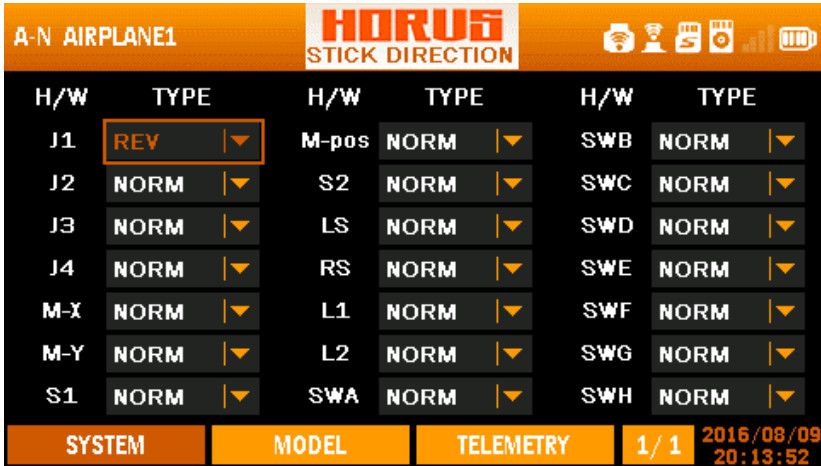
Overview of the stick direction menu screen
