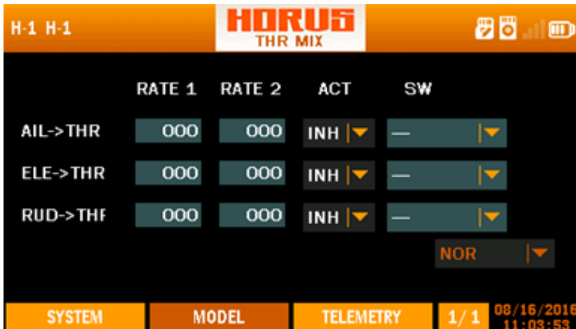
Overview of the throttle mix menu screen
